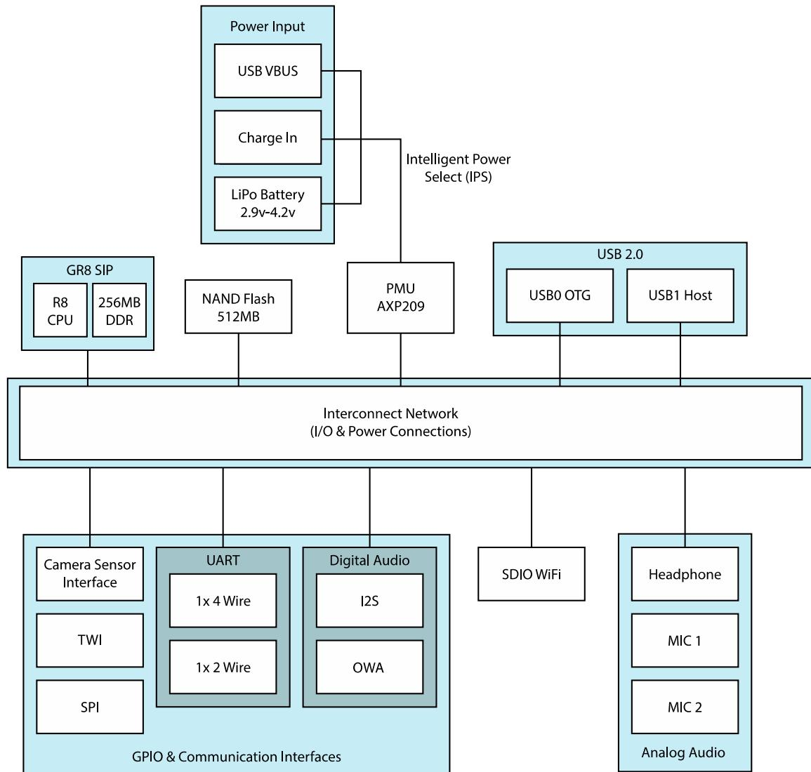
**Figure 3.1.: C.H.I.P. Pro Block Diagram**
