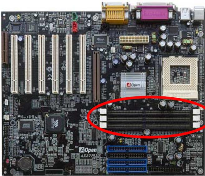
**Warning:** The AX37 Plus/AX37 Pro only supports DDR DRAM, please do not install the SDRAM on it, this will cause the memory sockets or DDR DRAM module damage.
