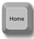
**Tip:** If your system hangs or fails to boot because of overclocking, simply use <Home> key to restore the default setting (433MHz) or you can wait the AOpen "Watch Dog Timer" reset the system after five seconds and system will auto-detect hardware again.
