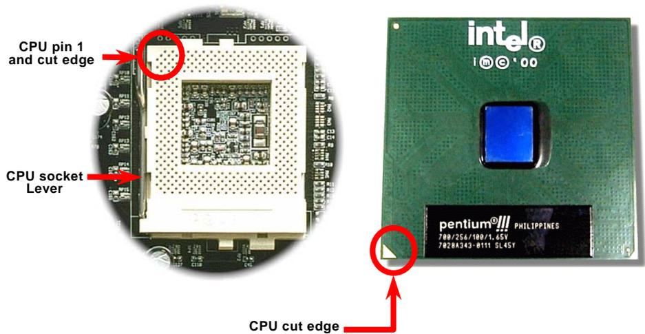
3. Press down the CPU socket level and finish CPU installation.
