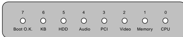
The total 8 LEDs light up alternatively if the system fails in one of eight stages. Once the LED7 (latest LED) is lit, this indicates that the system has completed its boot-up procedure.
