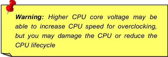
**Warning:** Higher CPU core voltage may be able to increase CPU speed for overclocking, but you may damage the CPU or reduce the CPU lifecycle
