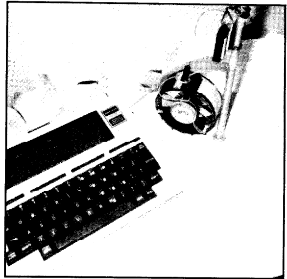
Photo 1. The author's Model 100, ready to measure air flow rate through the RS-232 port, is hooked up to his anemometer.
