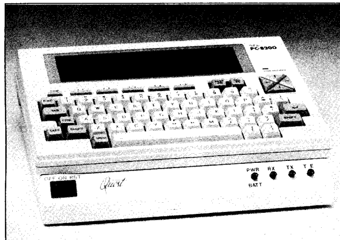
The QuEST provides wireless two-way digital communications between computers or computer peripherals.
