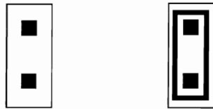
Figure B-2: Representation of disabled (left) and enabled (right) jumpers.
